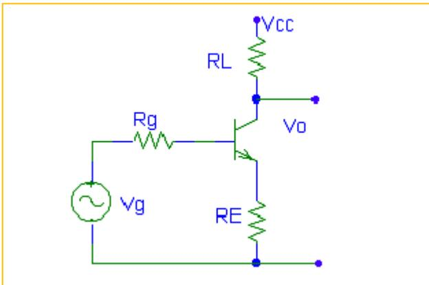
Transistor 2N929 operando en  $I_C = 4\text{mA}$ ,  $V_{CE} = 12\text{V}$ ,  $hie = 2200\Omega$ ;  $hre = 2 \times 10^{-4}$ ;  $hfe = 290$ ;  $hoe = 30 \times 10^{-6} \text{ mhos}$ ;  $R_L = 5000\Omega$ ;  $R_E = 100\Omega$ ;  $R_g = 500\Omega$ .
