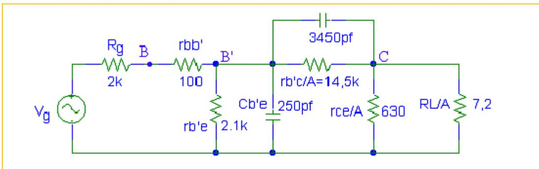
$$\text{como } \frac{R_L}{A} \ll \frac{r_{ce}}{A} \Rightarrow \frac{\frac{R_L}{A} \cdot \frac{r_{ce}}{A}}{\frac{R_L}{A} + \frac{r_{ce}}{A}} \approx \frac{R_L}{A}; \quad \frac{r_{b'c}}{A} \gg \frac{R_L}{A}$$
