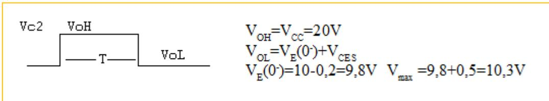
Tomando  $i_{C2}=10\text{mA}$ ,  $\beta=100$ ,  $i_{B2}>10\text{mA}/100=0,1\text{mA}$ .
