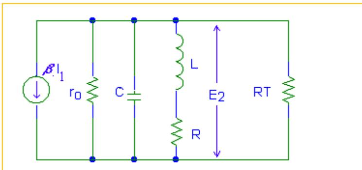
$$R_T = R_B \parallel R_i = R_{in} \quad E_2 = \frac{-\beta I_1}{\frac{1}{r_o} + \frac{1}{Z} + \frac{1}{R_T}}$$
