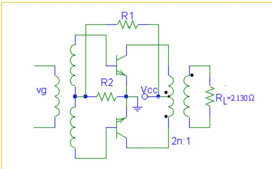
$$P_c = \frac{T_{jmax} - T_{max}}{\phi_{ja}} = \frac{175 - 70}{500} = 0,21W$$
