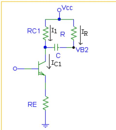
$$V_E(0^+) + V_\gamma - V_{B2}(0^+) = V_{CC} - V_{B2}(0^+) - (V_{CC} - V_{B2}(0^+))e^{-\frac{T}{\tau}}$$
