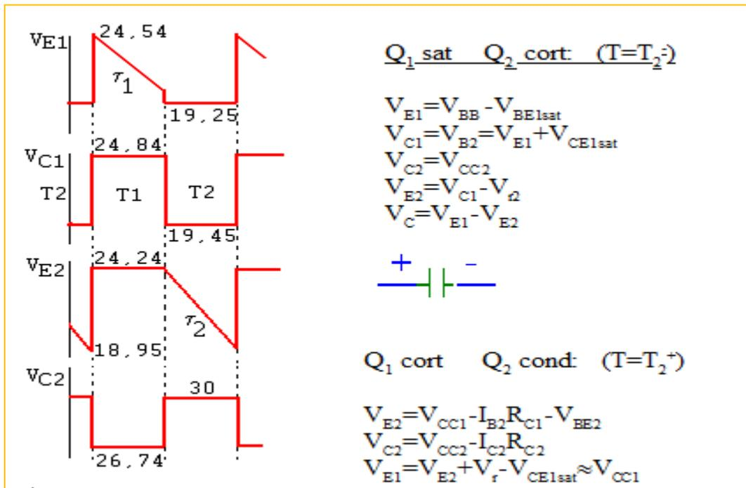
$$V_{E1} = V_{CC1} e^{-\frac{t}{\tau_1}} = V_{BB} - V_{\gamma 1}$$
