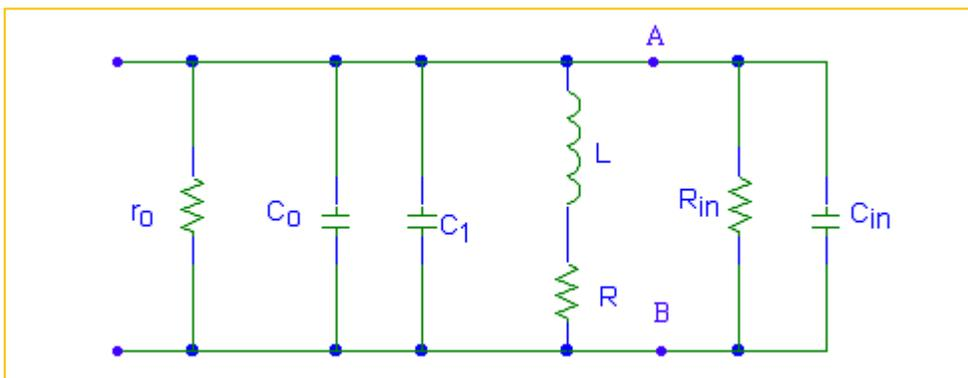
$$B = \frac{f_o}{Q_{ef}} \quad Q_{ef} = f_o/B = 500Kc / 10 Kc = 50 = (Q_o R_{sh}) / R_o$$
