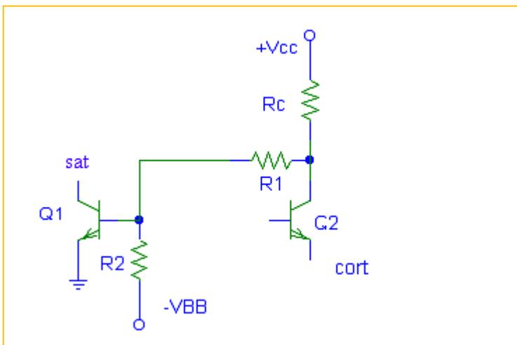
$$V_{C2} = \frac{V_{CC}R_1}{R_1 + R_2} + \frac{V_{BES}R_C}{R_1 + R_C}$$
