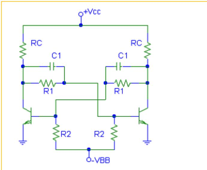
$$\tau = \frac{R_1 R_2 C_1}{R_1 + R_2};$$
