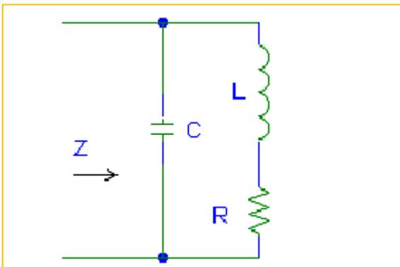
$$Z = \frac{\left(\frac{1}{j\omega C}\right)(R + j\omega L)}{R + j\left(\omega L - \frac{1}{\omega C}\right)}$$
