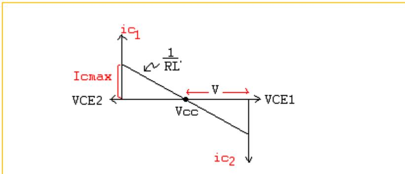
$$P_C = \frac{V_{CC}^2}{2R'_L} \left( \frac{2}{\pi} \times \frac{V}{V_{CC}} - \frac{V^2}{2V_{CC}^2} \right)$$
