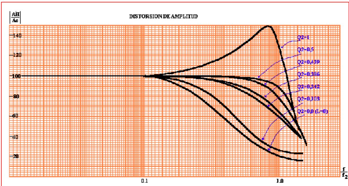
$$\phi = \text{ángulo de fase} \quad \phi = -\tan^{-1} \left[ \left( \frac{f}{f_2} \right) \left[ 1 - Q_2 + Q_2^2 \left( \frac{f}{f_2} \right)^2 \right] \right]$$
