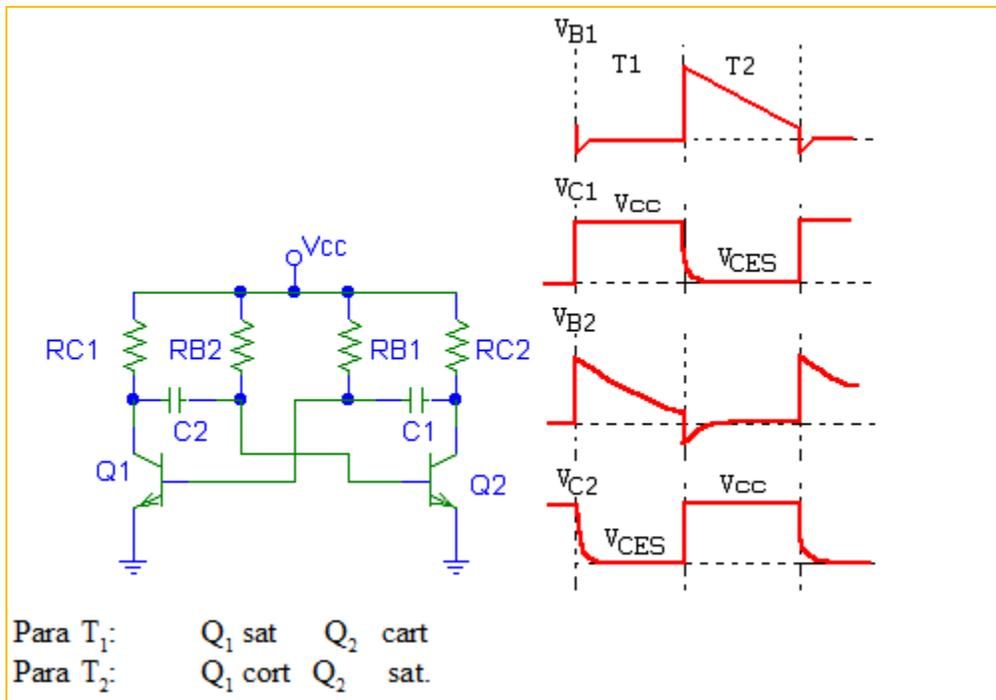
$$T_1 = 0,69 R_{B1} C_1 \quad T_2 = 0,69 R_{B2} C_2$$
