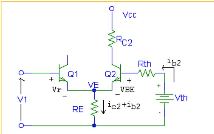
$$V_{th} = \frac{V_{CC}R_2}{R_{C1} + R_1 + R_2} = \frac{12(6)}{4 + 2 + 6} = 6V$$
