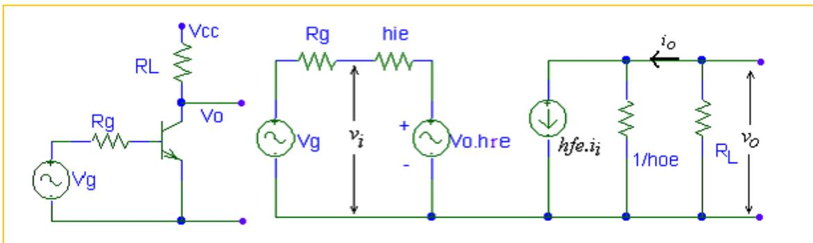
$$V_g = i_i R_g + i_i \cdot h_{ie} + V_o \cdot h_{re} \quad (1)$$
