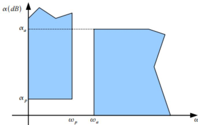
$$n = \frac{\log\left(\frac{10^{\alpha_a/10} - 1}{10^{\alpha_p/10} - 1}\right)}{2 \cdot \log\left(\frac{\omega_a}{\omega_p}\right)}$$
